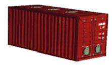
Frequent use: This container is designed for cargo in bulk. It gets loaded from the top. Suitable for chemical products, fertilizers, some flours, sugar, salt, plastic materials in lumps, etc.
