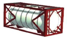
Frequent Use: Designed to transport liquids, hazardous substances such as toxic chemicals or corrosive, highly flammable subtances, oils, milk beer, wine, water, etc.
