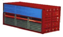
Frequent Use: similar to Open Top, but in this case it opens on the side. Suitable for big volume cargo that does not fit standard container doors. Perfect to load and unload in railway stations.
